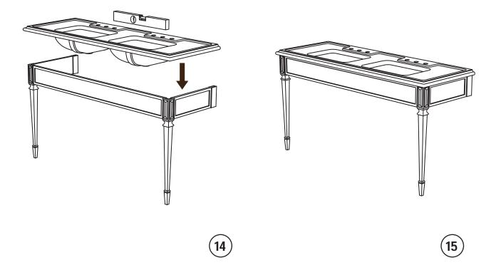
Carefully lower the countertop onto the batten and frame and position in place. Check with spirit level.
